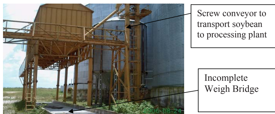
Connectivity between storage and processing plant
